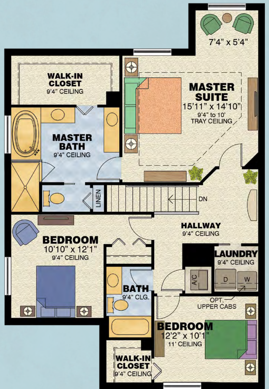
SECOND FLOOR PLAN
